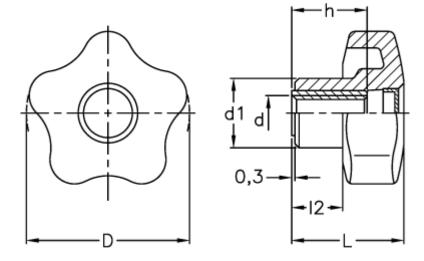
$$\begin{array}{ll} D & = 40 \\ d1 & = 17 \\ d \ 6H = M8 \\ h & = 18 \\ L & = 27 \\ l2 & = 12 \end{array}$$
